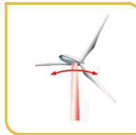
Axial tower oscillation
